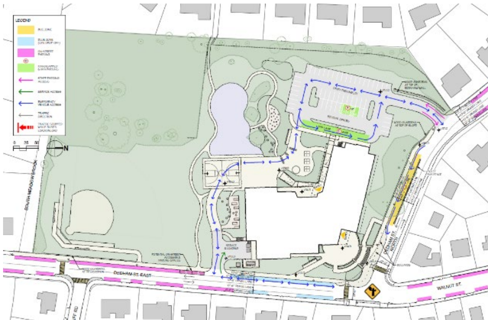
Left: Existing school traffic design provided by DiNisco Design. Bus loading areas shown in yellow and pick-up/drop-off in blue.
