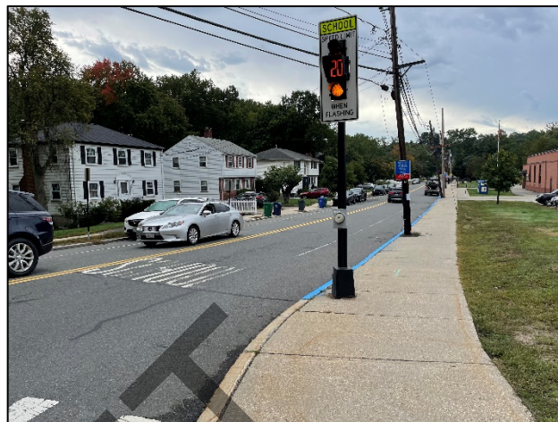
Photo 8: Flashing school zone speed limit signs at the beginning of “blue zone”
